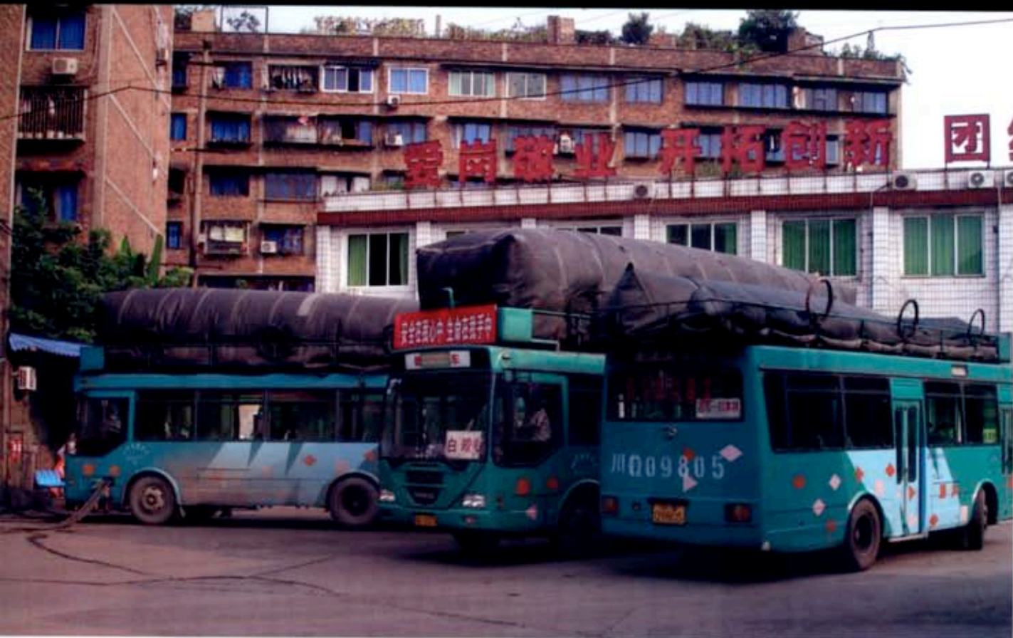
Buses in the town of Gong Xian, China, equipped to run on captured methane from the Baijiao mine.
